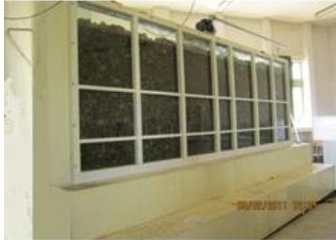
Fig. 3. Schematic of the permeameter.
