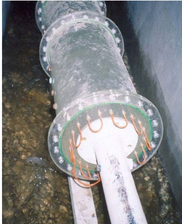
Fig. 2. Picture of sudden pipe expansion
