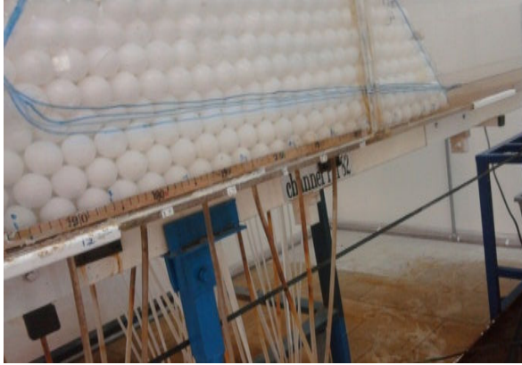
Fig. 3. Dam model with the same size diameter materials (Diameter = 37 mm) with inbuilt spillway on the upstream face
