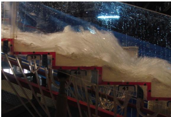
Fig. 4. Step with slope of 7^\circ , end sill height of 6 mm and thickness of 5 mm
