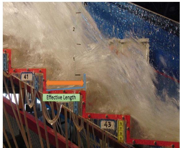
Fig. 8. Step with slope of 10°, end sill height of 10 mm and thickness of 5 mm
