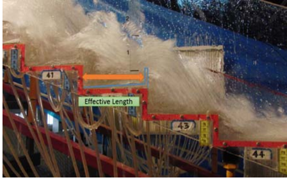
Fig. 9. Step with slope of 10°, end sill height of 10 mm and thickness of 10 mm
