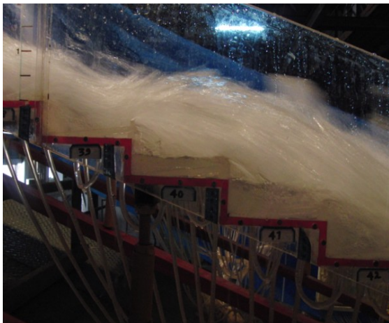
Fig. 14. Step with slope of 7°, end sill height of 6mm and thickness of 5mm
