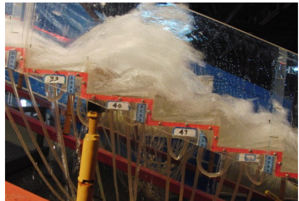
Fig. 5. Step with slope of 12^\circ , end sill height of 15 mm and thickness of 5 mm
