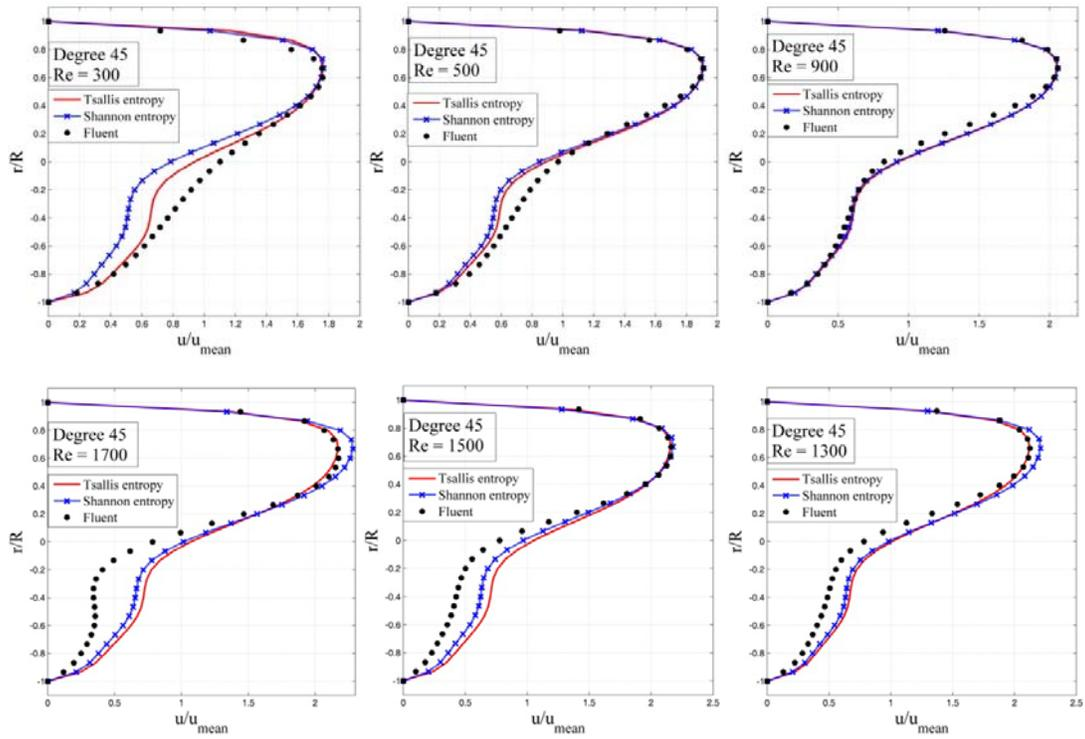
Fig. 5. Velocity distribution in deviation angle of 45 degrees
