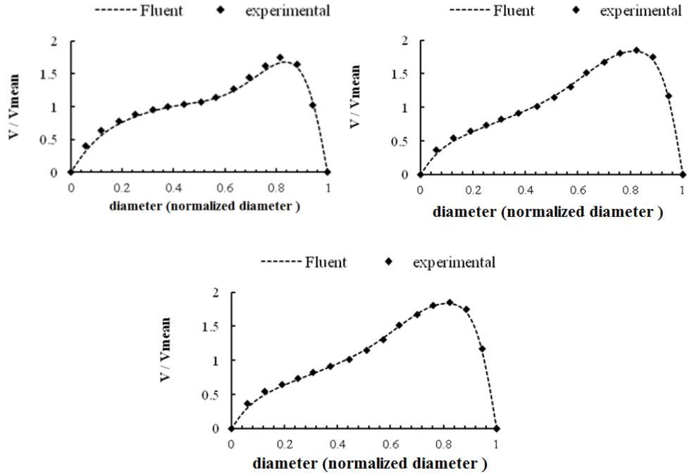
Figure 2. Comparison of numerical modeling velocity profiles and experimental results of (Olsen et al) at Reynolds number 300
