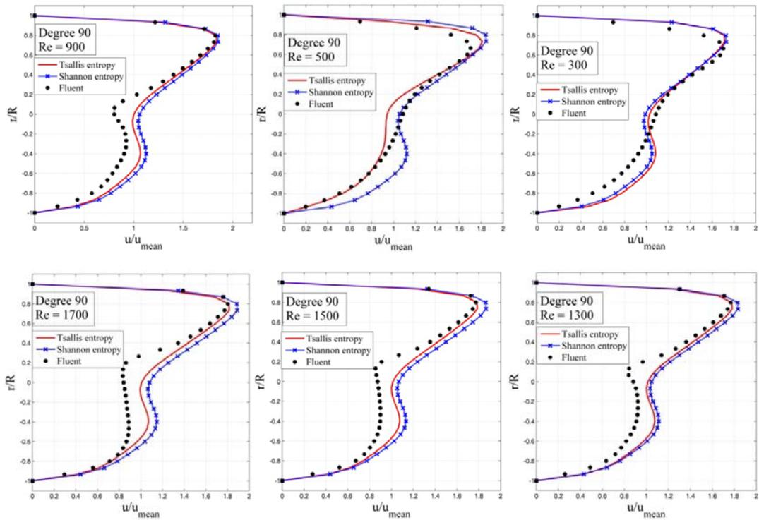
Fig. 6. Velocity distribution in deviation angle of 90 degree
