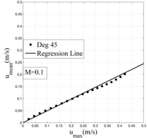
Fig. 3. Linear relation between average velocity and maximum velocity at the 45-degree bend
