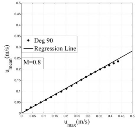
Fig. 4. Linear relation between average velocity and maximum velocity at the 90-degree bend
