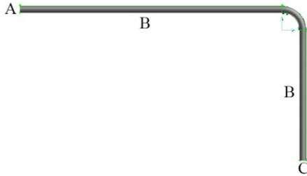
Figure 1. Boundary conditions and geometry of the 90-degree bend
